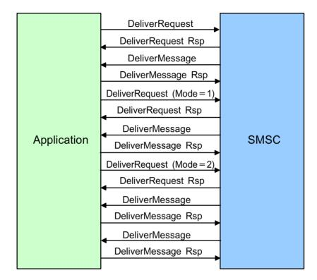
Figure 2. Flow of delivery request operations
